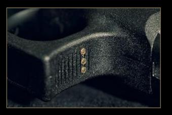
3 pins connect the laser to the trigger safety circuit.
